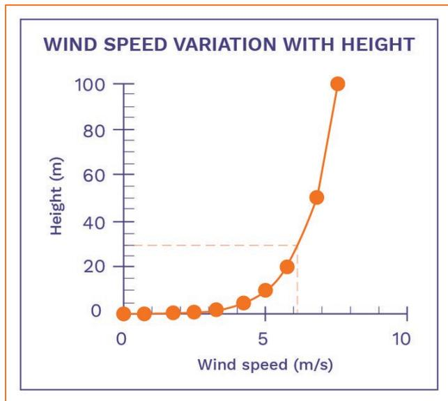
Figure 5-3: Example of a wind speed gradient
