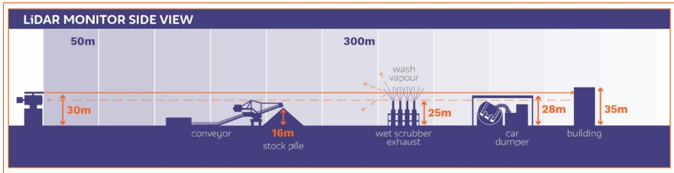
Figure 5-1: Example of LiDAR scan height with various potential sources within the airshed
