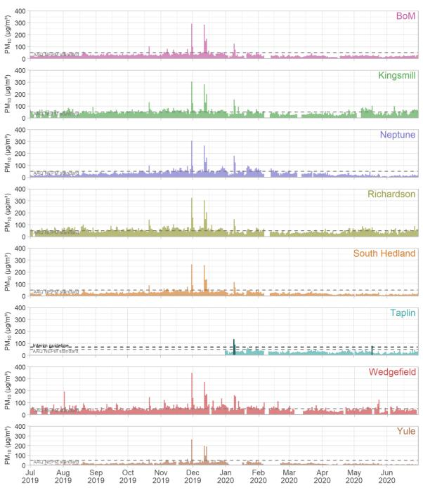
Figure 4-1: FY 2019/20 time series plots of 24-hour average concentrations of PM<sub>10</sub>
