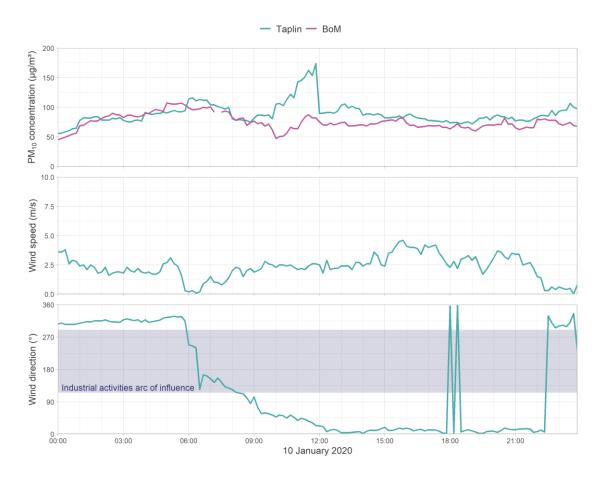
Figure 7-5: Time series of concentrations of PM<sub>10</sub> at Taplin and BoM (top) and wind speed at Taplin (middle) and wind direction at Taplin (bottom) on 10 January 2020
